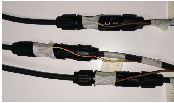
Couple 1 Photo during temperature test – Thermocouples applied on case of connector The samples provided are all the same n.3 samples (male-female combination) identified 1A - 2A - 3A during the tests. Cable length 1400mm - 6mm 2
