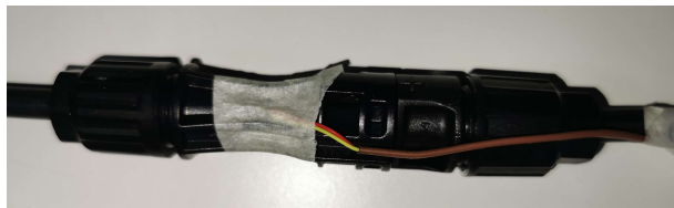
Couple 2 Photo during temperature test – Thermocouples applied on case of connector The samples provided are all the same n.3 samples (male-female combination) identified 1A - 2A - 3A during the tests. Cable length 1400mm - 6mm 2
